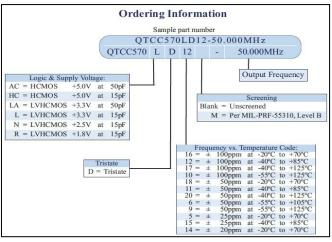
VCC1-B3B-FREQ = QTCC570LD18-FREQ VCC1-F3D-FREQ = QTCC570LAD11-FREQ VCC1-B3R-FREQ = QTCC570LD9-FREQ VCC1-E2F-FREQ = QTCC570ACD15-FREQ
