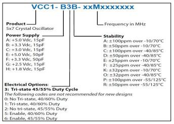
Any Vectron Electrical Option cross to Q-TECH "D" Vectron VCC1 does not have a Screen option
